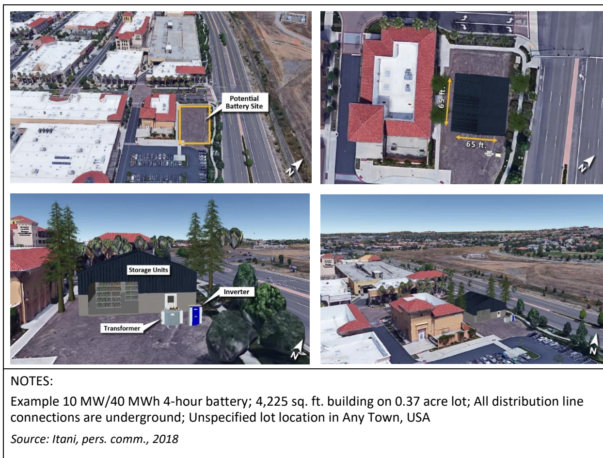
Figure 3-1513. Example Energy Storage Facility Enclosed in Building
